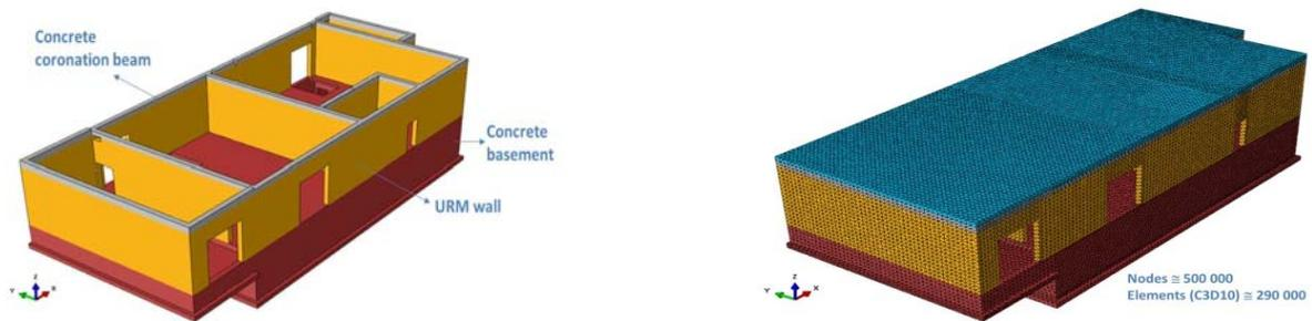
Figure 3. FE meshing of the numerical model.
